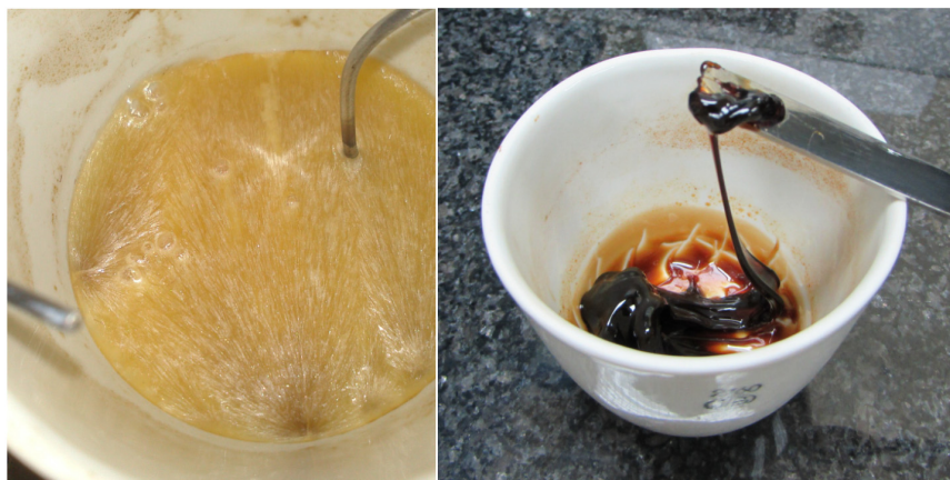
Figure 2. D-mannitol appearance after being kept at 180 °C under air (left) during 12 h and (right) during 166 h.
