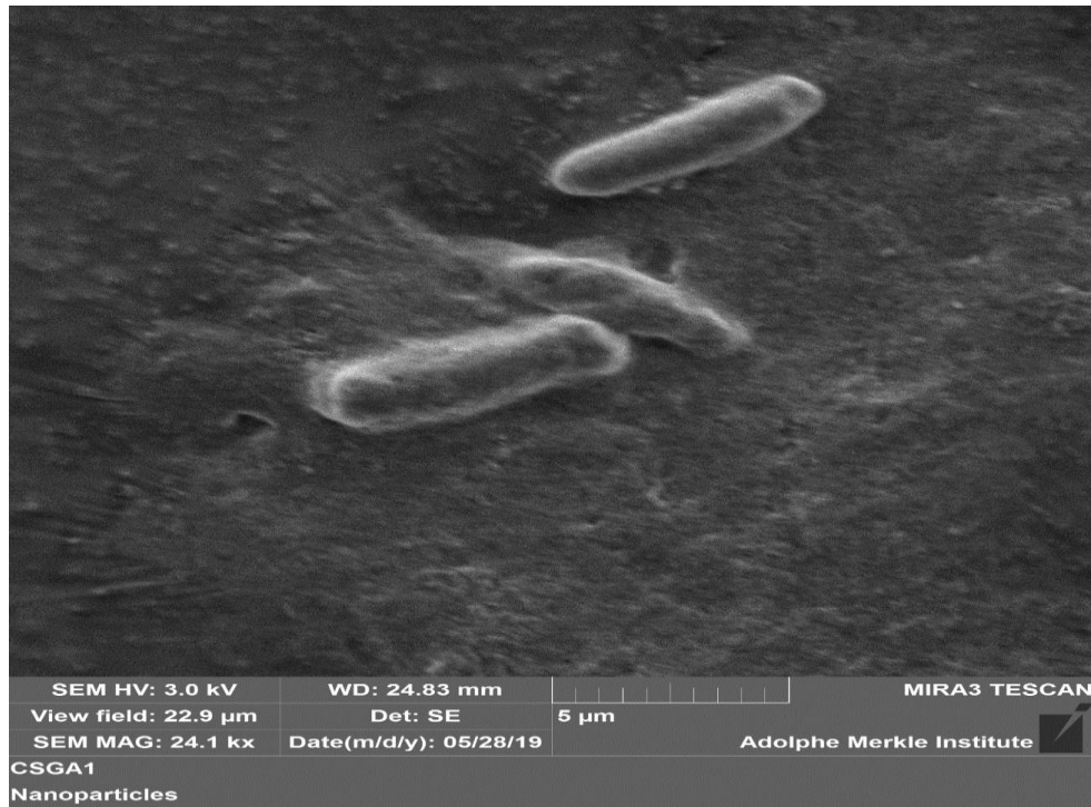
Figure 3. Showed nanoparticles based on chitosan encapsulating aqueous extract from garlic and onion, nanoparticles characterized by rod-shape.
