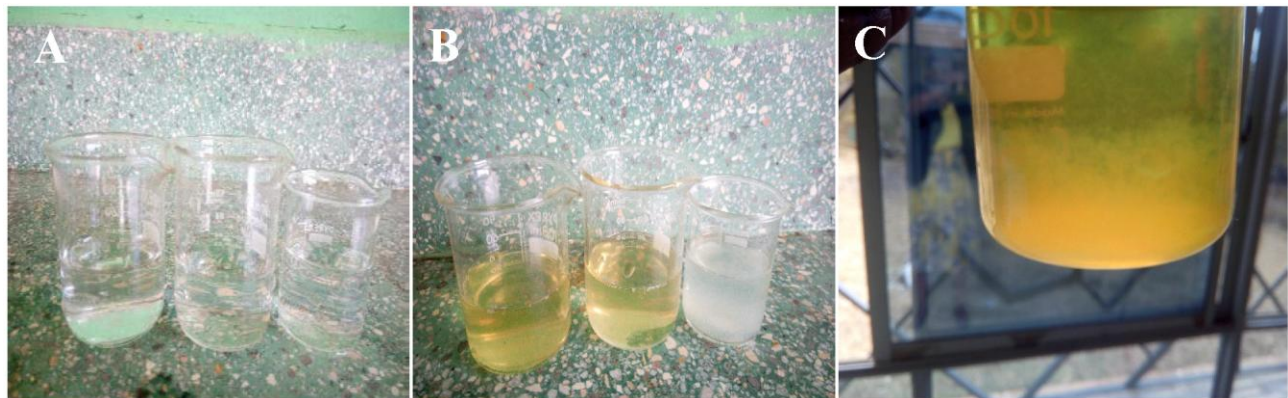
Figure 1. PH sensitivity of chitosan nanoparticles of garlic and onion. (A) Chitosan nanoparticles of garlic and onion in water. (B) and (C) are the increased of the pH with 300 \mu l of NAOH solution, from pH 4 to 8.
