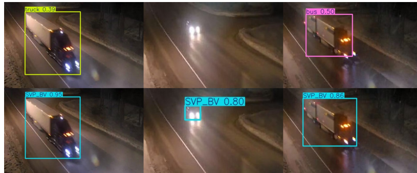
Figure 6. Comparison of predictions for single-vehicle images with ambient light (Top row: Original YOLO11 model; and bottom row: fine-tuned YOLO11 model).
