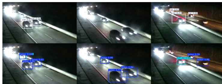
Figure 7. Comparison of predictions on multiple-vehicle images without ambient light (Top row: Original YOLO11 model; and bottom row: fine-tuned YOLO11 model).
