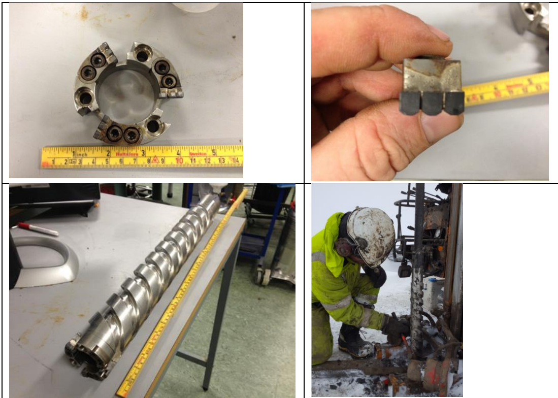
Figure 6 The SINTEF permafrost corer; drill piece (top left), PCD inserts (top right), frost corer assembled (lower left) and sampling in Adventdalen (bottom right).
