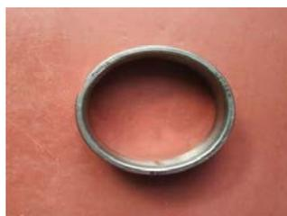
**Figure 9.** Early fault bearing.
