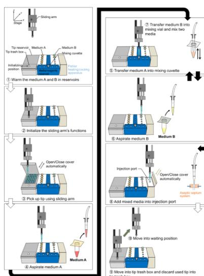
**Supplementary Figure 6.** Schematic showing how the robotic arm for liquid handling supply culture medium in chip.
