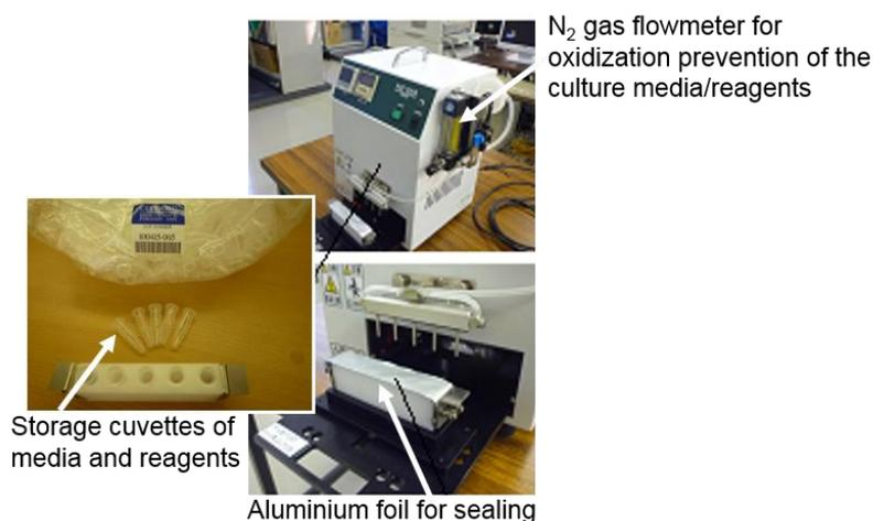
**Supplementary Figure 1.** Photograph of the aluminum foil sealing machine for storage of media and reagents.
