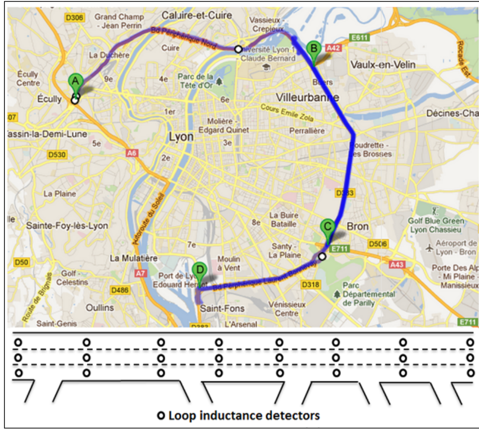
FIGURE 3. Test site section (B → C) divided into 7 cells and its detector configuration
