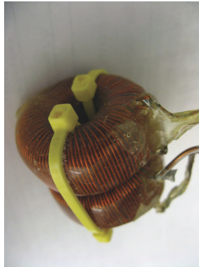
FIGURE 5. Salinity sensor coil arrangement.
