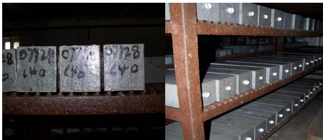
Figure 2. Specimen casting and curing.
