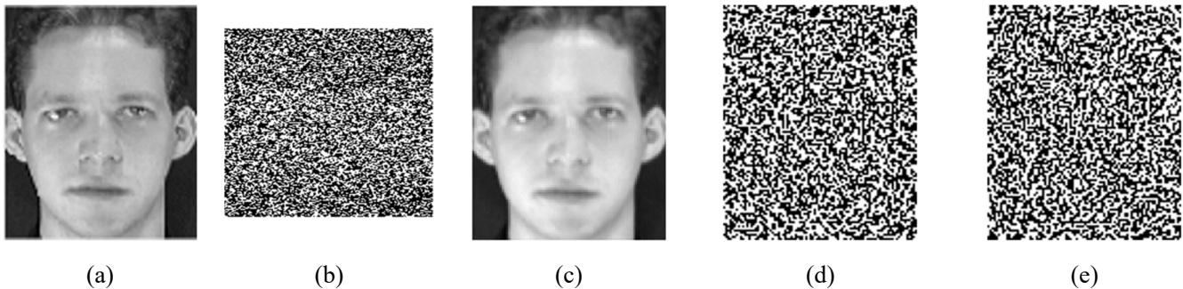
Figure 7. The sensitivity testing of the encryption algorithm. (a) Original image, (b) Encrypted Image, (c) Decrypt correctly, (d) Decrypt incorrectly ( x_0 = 0.36 + 10^{-16} ), (e) Decrypt incorrectly ( a = 1.4 + 10^{-16} ).
