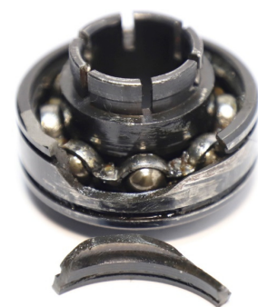
(c) Outer race fracture
