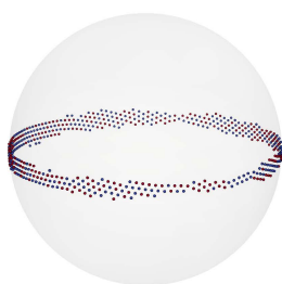
Figure 3. Particle distribution at t = t_f for N = 512 particles with E = 200V/mm . The damping parameter \chi = 1.0 .
