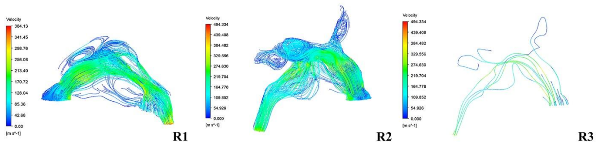
Figure 6. Streamline diagram of normal and Draf III model. R1: Streamline of normal model (Left View). R2: Streamline of Draf III model (Right View). R3: Streamline of Draf III model by simulating a small amount of air input from the inlet (Right View).
