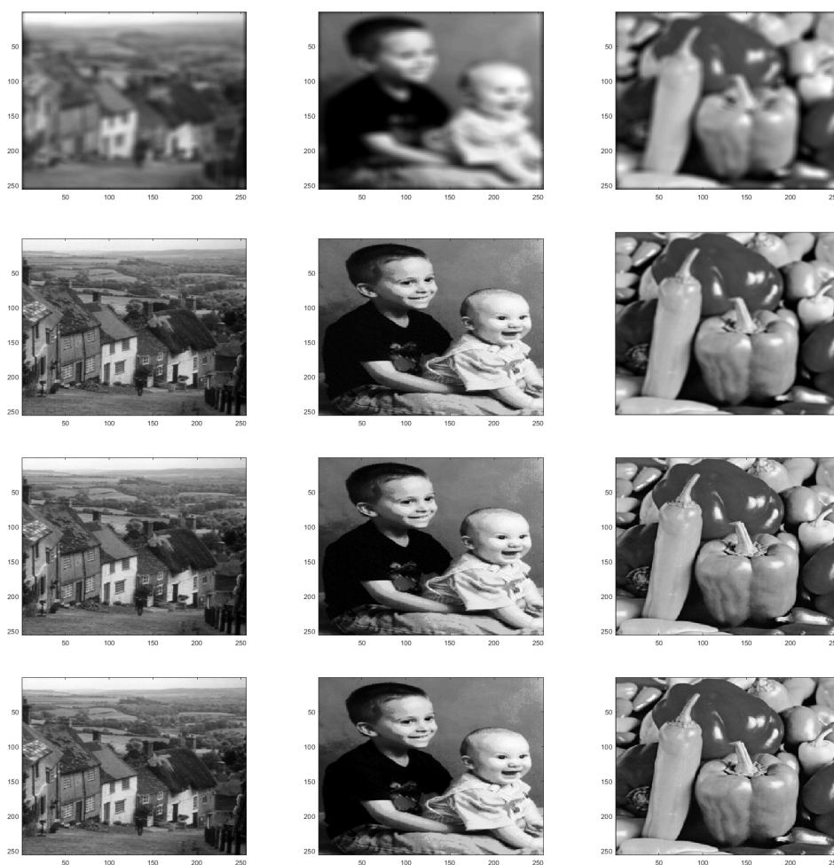
Figure 5. (first row) Blurry images, (second row) TVM deblurred images, (third row) ALM deblurred images and (last row) PALM deblurred images.
