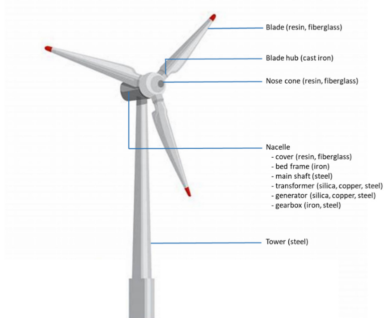
Figure 2. Wind turbine components and main materials (authors’ own creation).
