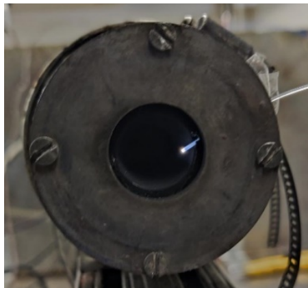
(c) Fiber-optic cable installed at nozzle exit plane
