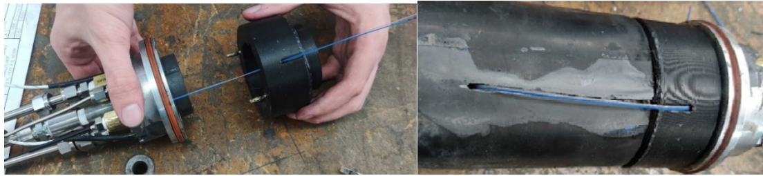
(a) Fiber-optic interface to injector/ ignitor caps (b) Fiber-optic cable installed in fuel grain
