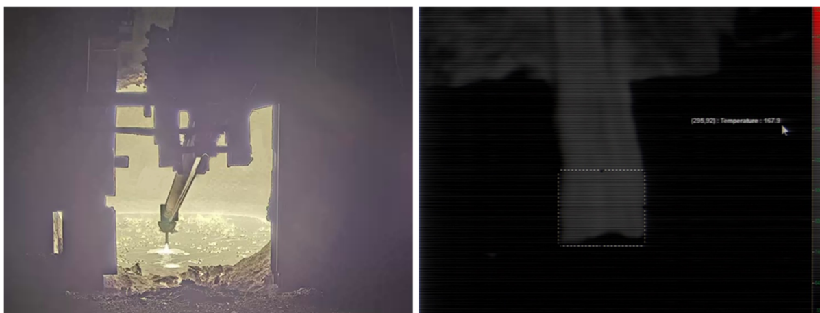
Figure 9. Sample images of dart injection (left) and tapping stream from BOF (right).
