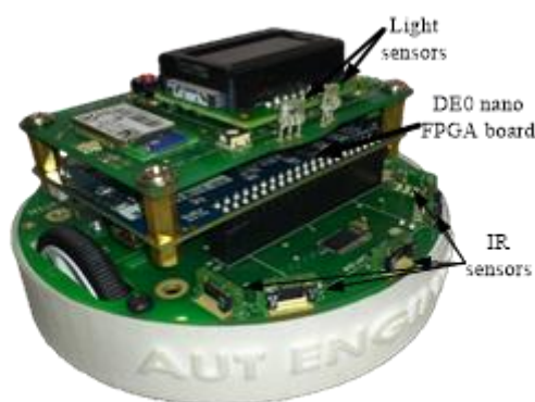
Figure 2. The physical two wheeled robot that was designed at the Auckland University of Technology for future research in the reality gap between simulation and real world.
