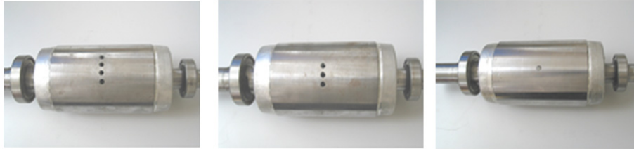
Figure 9. Emulation of the broken bar fault.
