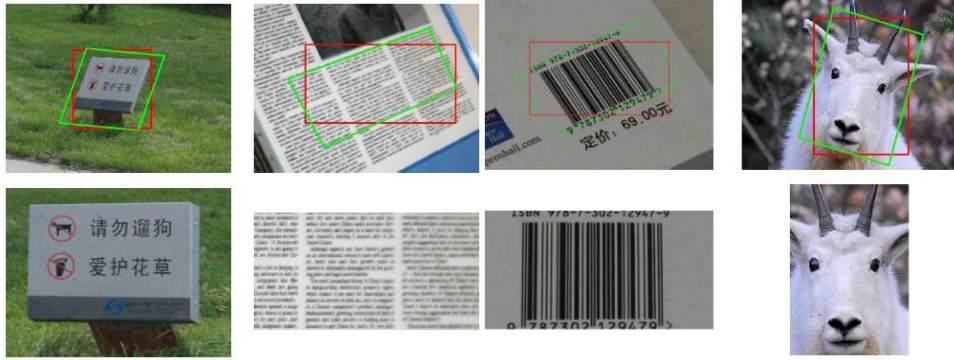
FIGURE 6. Example of using TILT for image rectification, adapted from [78]. The first row are the original image patches (in rectangles) and their respective rectification transformations (in quadrilaterals). The transformations are to map the quadrilaterals into rectangles). The second row are the rectified image patches.
