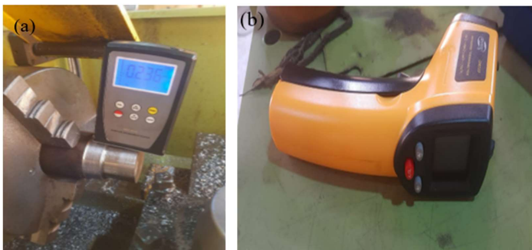
Figure 4. Measurement devices used in the experiment: (a) roughness test of the workpiece during turning operation, (b) photographic view of infrared thermometer.
