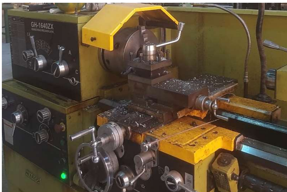
Figure 2. Pictorial view of GH-1640ZX model Lathe machine used for machining.
