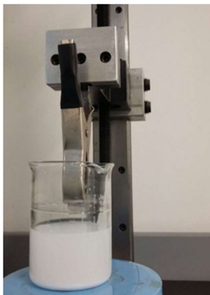
Figure 1. Coated samples by the immersion-removal process at inlet velocity of 10 mm/s.
