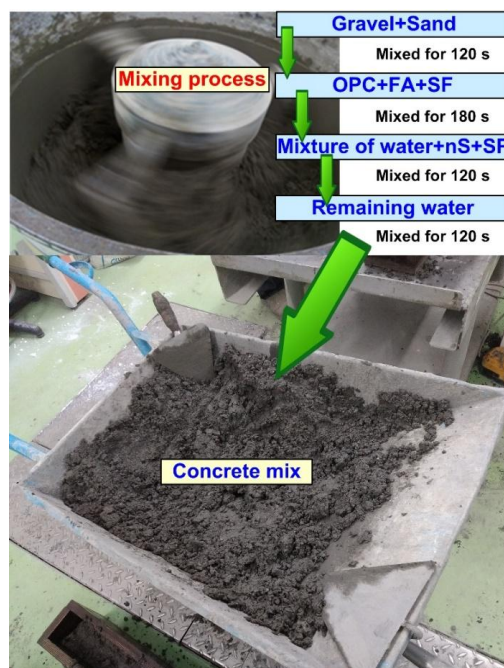
Figure 1. Full mixing process of concrete made by combined SCMs with OPC.
