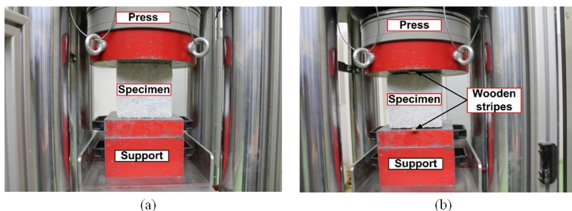
Figure 2. Specimens during the compressive strength (a) and splitting tensile strength (b) tests.
