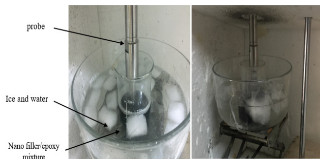
Figure 2. Ultra-sonication of the nano filler/epoxy mixtures.
