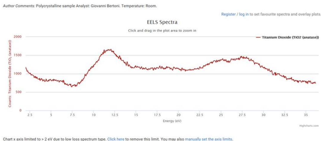
Figure 8. EELS spectra of \text{TiO}_2 referred from EELS data base [31].
