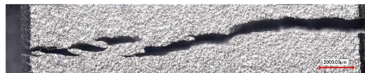
(a) Non-peened ( \sigma_a = 224 MPa, N = 510,300 )
