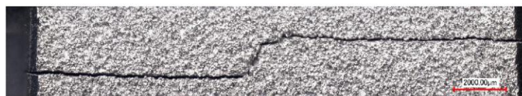
(b) Cavitation peened ( \sigma_a = 328 MPa, N = 319,300 )
