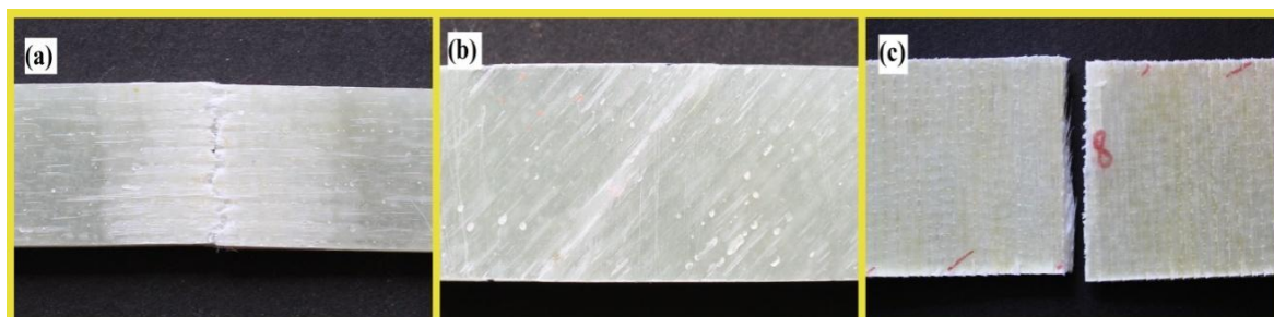
Figure 7. Failure regions of the tested samples (composite-D) under interlaminar shear loading at: (a) longitudinal direction, (b) 45^\circ fiber orientations and (c) transverse directions.
