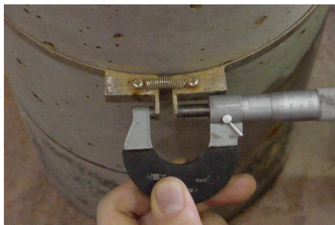
Figure 4. A typical mechanical expansion collar.
