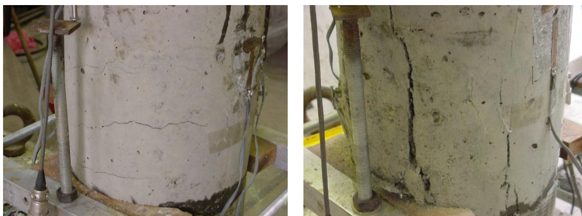
Figure 13. Cracking of corroded M-DFRCC column during structural test (left) and after failure (right).
