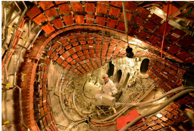
Figure 2. Internal view of Plasma Vessel with basic types of Plasma Facing Components.
