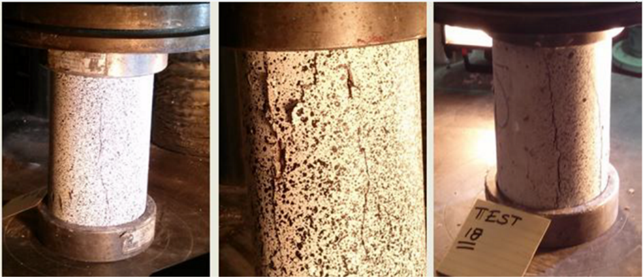
Figure 3. Mortar specimen inside Tinus Olsen test frame.
