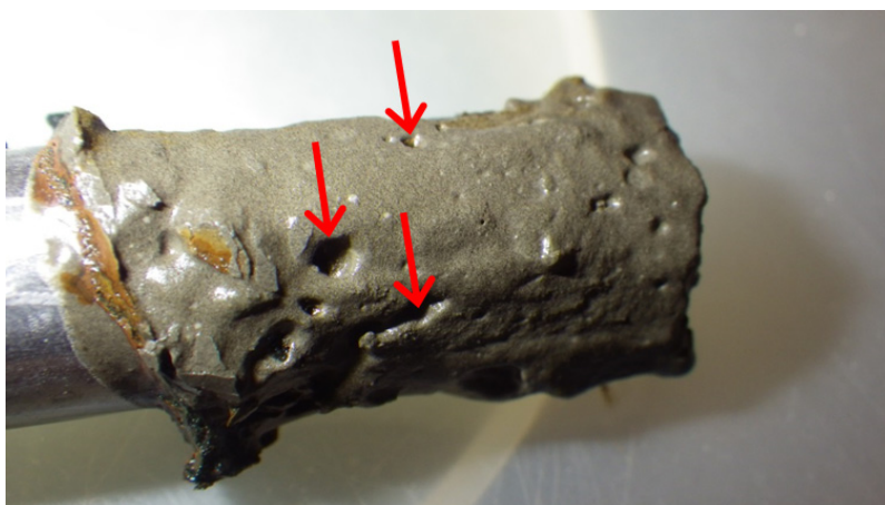
Figure 4. Voids (presumably created by oxygen bubbles) in the cement bonded to the positive electrode.
