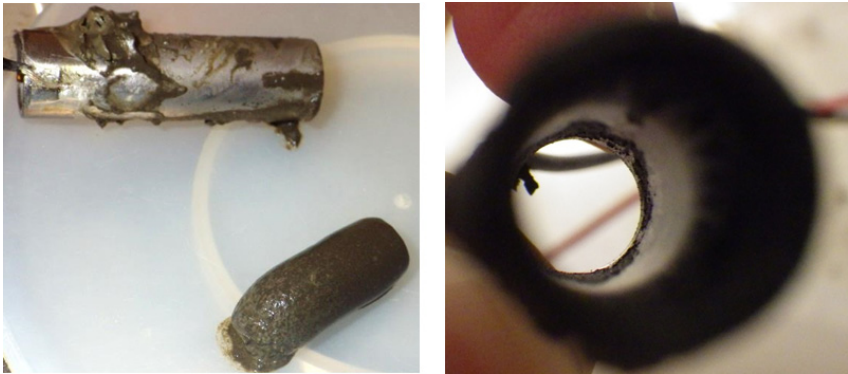
Figure 8. Poor bonding at the negative electrode: cement column fell out of the pipe when the pipe was pulled out of the slurry.
