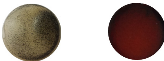
Figure 4. Side-by-side comparison of 1 wt% C_{60} incorporated into a TE matrix using pure C_{60} (left) and C_{60}(\text{TMB-PPO})_5 (right).
