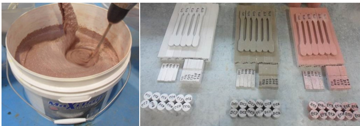
Figure 1. Preparation of specimens. (a) mixing of the grouts and (b) part of typical test specimens.
