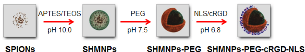
Figure 11. Scheme of the synthetic route of amine-functionalized silica coated SPIONs (SHMNPs) surface functionalization (a nuclear localization sequence (NLS) and integrin-ligand (cRGD)). Reproduced with permission from [103] © 2015, Wiley-VCH.
