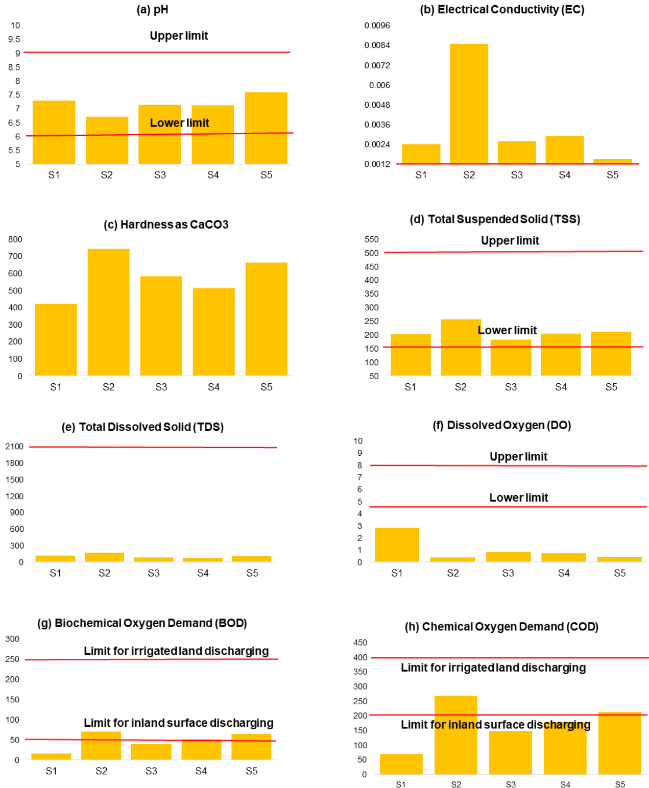
Figure 2. Changes in (a) pH; (b) Electrical Conductivity (EC); (c) Hardness as CaCO 3 ; (d) Total Suspended Solid (TSS); (e) Total Dissolved Solid (TDS); (f) Dissolved Oxygen (DO); (g) Biochemical Oxygen Demand (BOD 5d at 20 °C); (h) Chemical Oxygen Demand (COD) at different sampling location.
