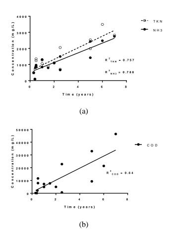
**Figure 4.** The relation between: (a) nitrogen concentrations (dashed line showing TKN, solid line showing ammonia); and (b) COD in faecal sludge sampled from the pits versus pit emptying time interval.
