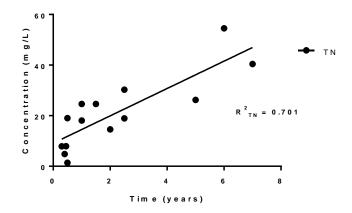
**Figure 5.** Total nitrogen concentrations in wells versus emptying time interval of the closest latrine; data shown are from the wet season sampling round.
