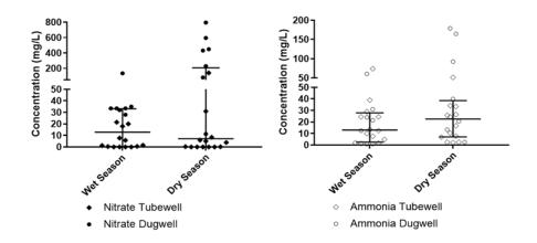
**Figure 2.** Whisker plots showing nitrate and ammonia concentrations in tube wells and dug wells in the wet and dry seasons, combining data from all three case study sites.
