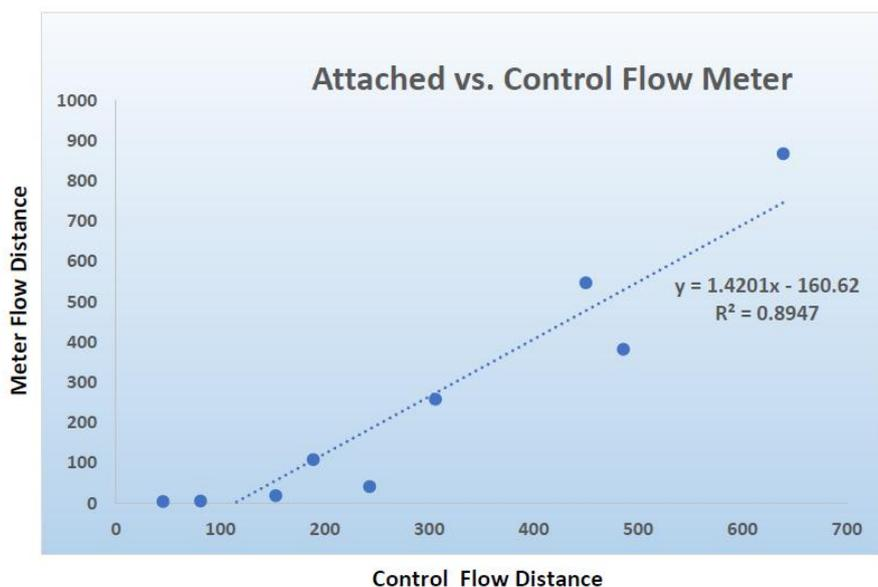
**Figure 3.** Regression analysis showing relationship of attached flow meter distance calculation versus hand held control meter distance.
