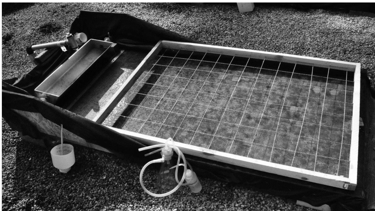
Figure 2. Photography of the ATS with the inflow and tipping bucket at the left side and the constructed sampling grid above the flow lane.
