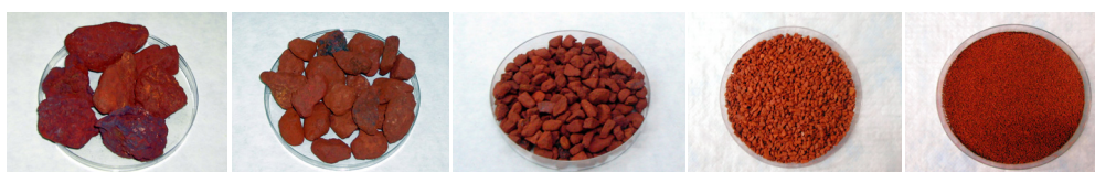
Figure 1. Hematite particles of iron ore with different sizes used in laboratory experiments and industrial scale tests.
