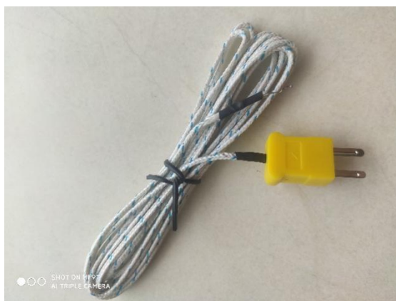
Figure 6. K-type probes used to measure temperature.
