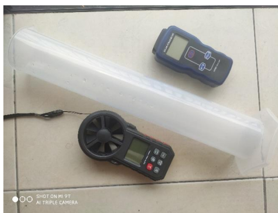
Figure 7. Tools used for measuring air speed, solar radiation and productivity.
