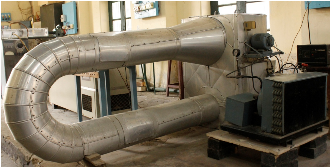
Figure 1. U-Duct for forced convection cooling.
