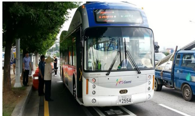
Figure 14. Olev kiast dynamic charging-South Korea [41].
