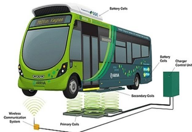
Figure 13. Inductive charging system [38].
