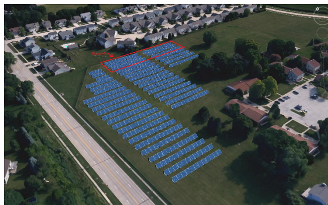
Figure 3. 3D rendering of Center for Renewable Energy ground mounted PV system (phase one system size outlined in red color).
