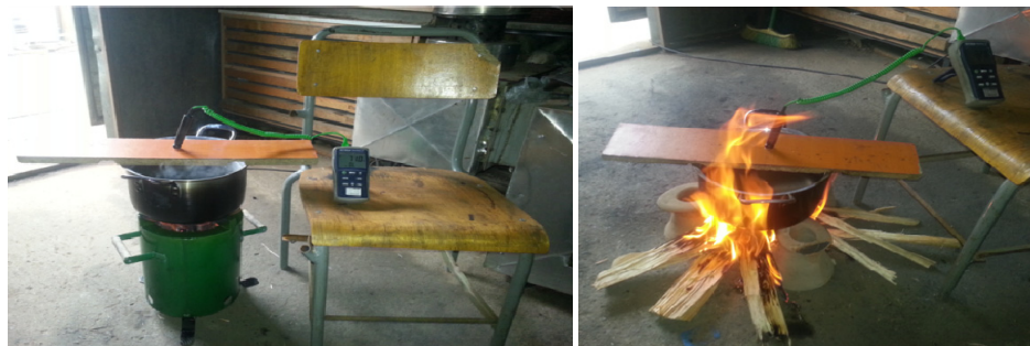
Figure 2. Test set-up of micro-gasifier and open-fire stove.
