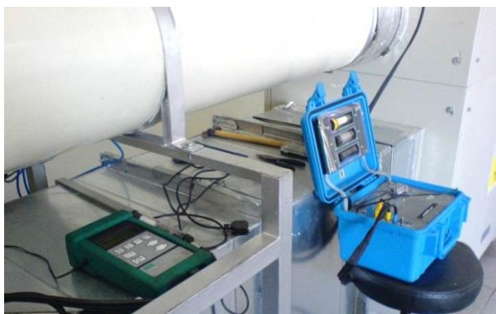
Figure 4. Two gas analyzers connected to the microturbine.
