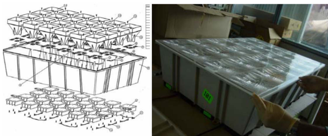
Figure 2. PhoCUS CPV module schematic view and picture.
