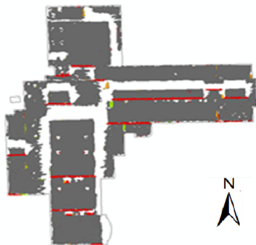
Figure 8. Example of south-facing (red) and flat (gray) roof space on the same building based on the GIS analysis.
