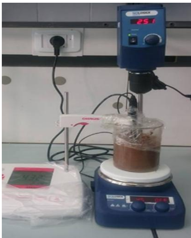
Figure 1. Controlled fermentation tank tested on a laboratory scale.
