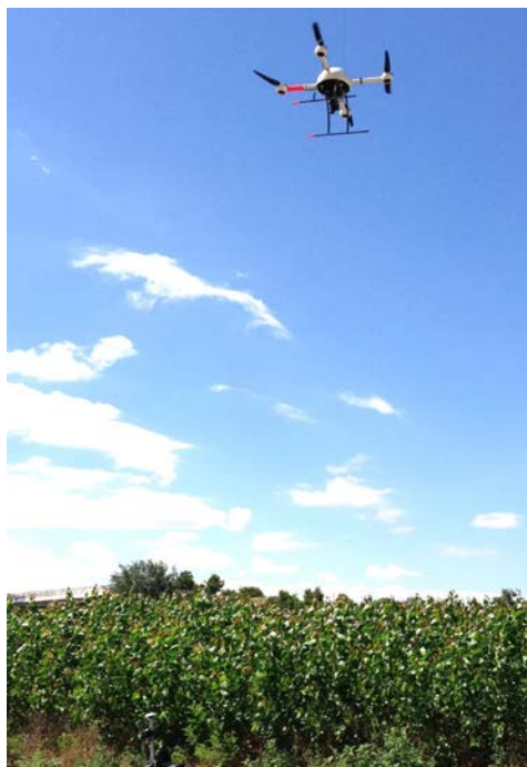
Figure 2. The UAV with the multi-spectral camera flying towards the poplar plantation.
