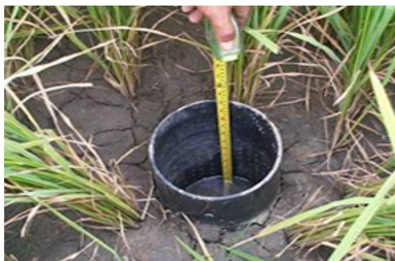
Figure 1. Perched plastic tube and steel tape. Source: IRRI
